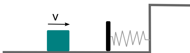
FIG. 2: Toy-train stopped by spring compression.
